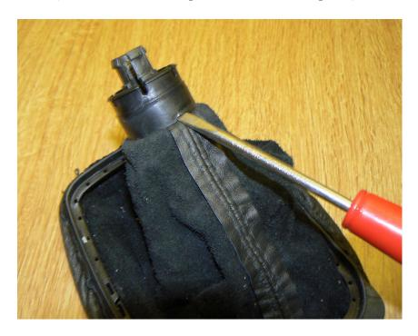
Take note of how the gaiter / metal ring is arranged.
