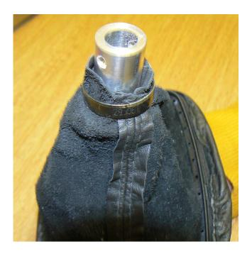
Fit the gaiter securing collar and tighten the grub screw. Make sure it is pushed down tightly against the gaiter.
