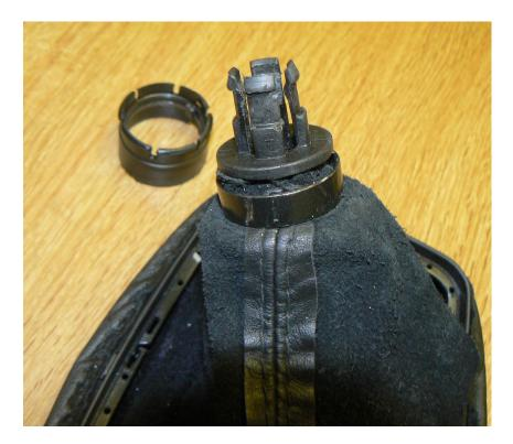
Transfer gaiter & metal ring to the pool ball knob. Make sure you have the frame orientated the same way as on the original gear knob, otherwise you may later find the pool ball faces the wrong way.
